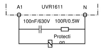
With outputs 5, 12 and 13, care should be taken to ensure that these are always potential free and carry no live voltage. Direct switching of a 230V consumer is therefore only possible with the appropriate wiring.
