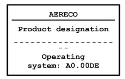
**Operating system:** Unit software version number. The latest software (higher number) can be downloaded from <a href="https://www.ta.co.at/en/">https://www.ta.co.at/en/</a>. It can be transferred to the controller boot loader via an add-on device.
