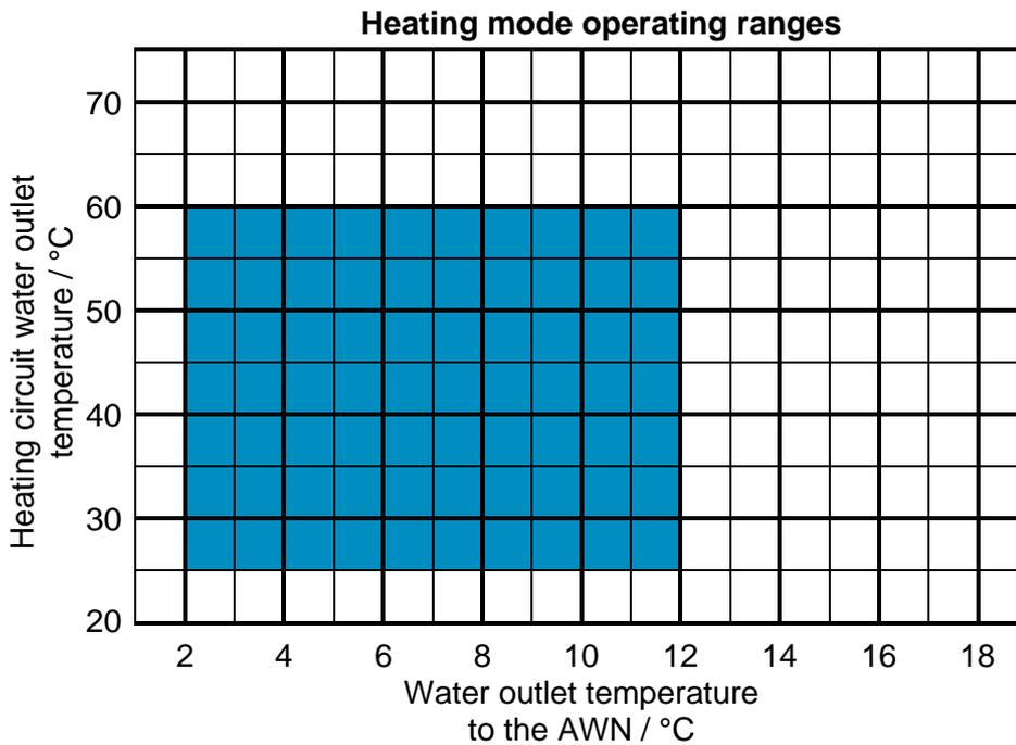
When operating under full load, the Connect WP provides hot water up to  $60^\circ\text{C}$ . An efficiency limit is pre-programmed at the factory, which switches off the heat pump at a buffer memory temperature of  $45^\circ\text{C}$  (bottom). This can be adapted on site or during commissioning. This is particularly suitable for operation with own electricity (e.g. from photovoltaics). Please refer to the technical documentation for further details.
